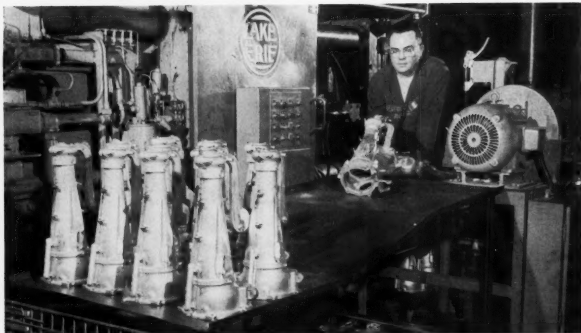
IN PRODUCTION: Aluminum transmission housings are made at Ford plant using hot metal from Reynolds.
